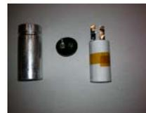
Can, header, and spiral wound electrode-separator bobbin
