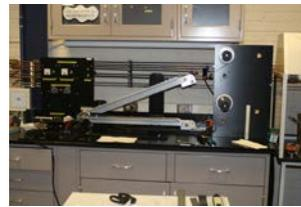
Electrode coating machine (left) and bobbin winder (right).
